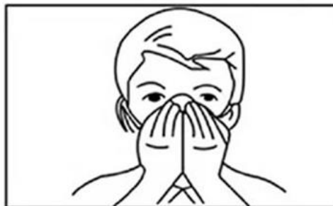
5. Check mask tightness before entering work area . • Cover your face with both hands and exhale quickly • If air leaks from the nose, go back to step 4 • If air leaks from the edges, adjust the earband
